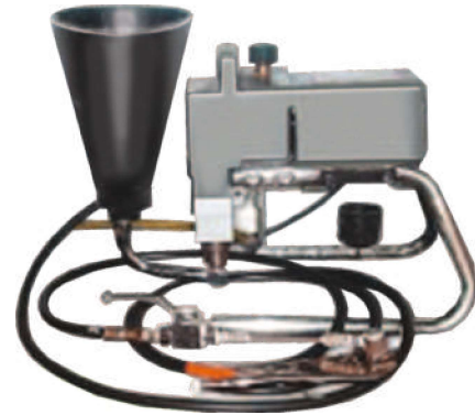
Typical Injection Pump
